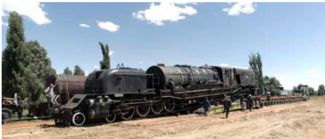
Unloading GMA/M 4079 at Sandstone from the multi axle trailer. A lowbed gooseneck trailer is being used as an unloading ramp. An innovation introduced by Mercor during the move of the Sandstone locos from Bloemfontein. Pictures by Ron Nell.
