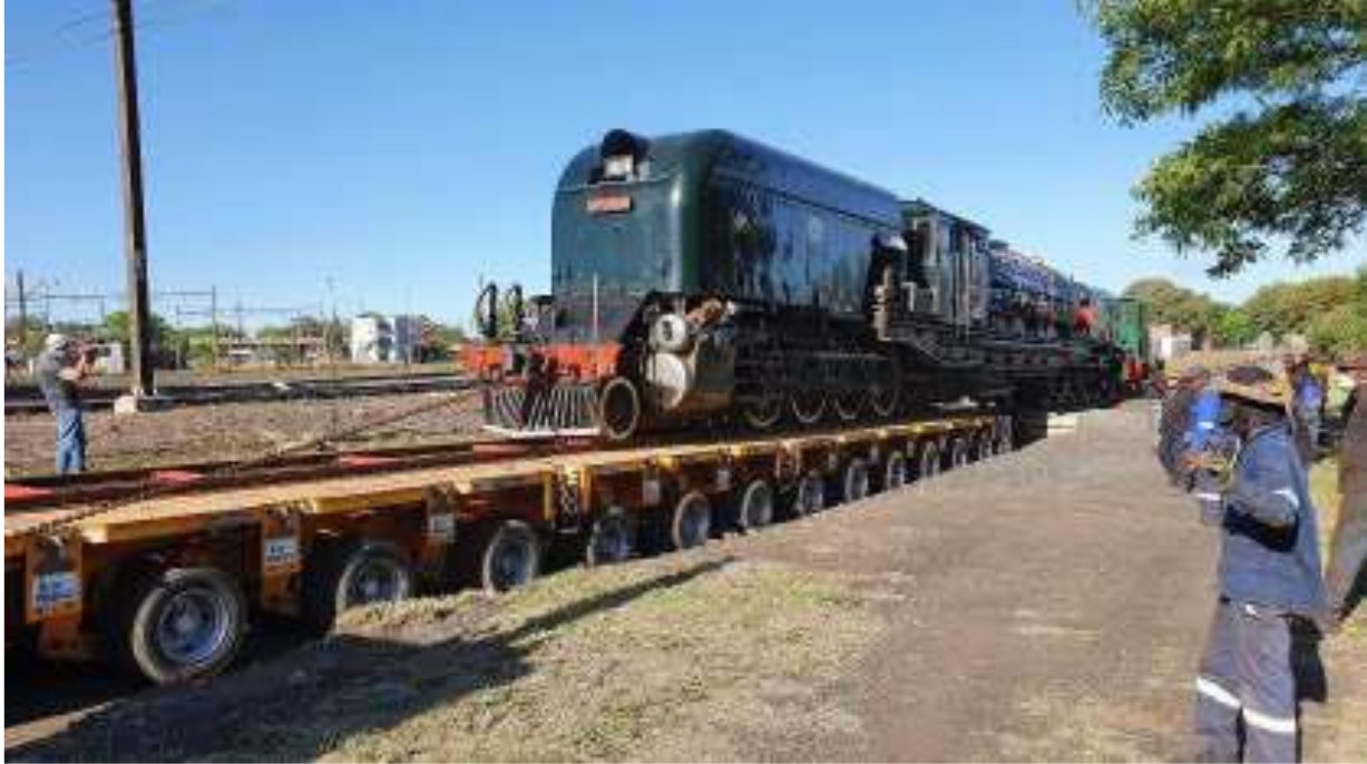
GMA/M 4079, "Lyndie Lou" is winched on to the multi axle trailer. At 154000kg, just too much for the mighty Hunslet! Picture by Sandstone Heritage Trust.
